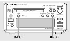
Even if your recording source is not Onkyo **RI**-compatible, you can perform synchronized recording. You can also make signal synchro recording from a connected CDR-201A.
